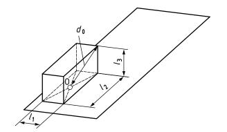
a) Reference box on one reflecting plane,  $d_0 = \sqrt{(l_1/2)^2 + (l_2/2)^2 + l_3^2}$
